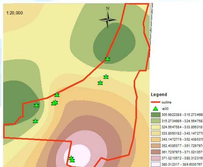
Figure 4. Average shear wave velocity for the top 30 m depth
