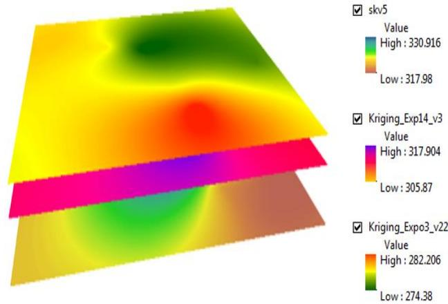
Figure 5. Mapped 2D shear wave velocity layer models at different depths for the IITM campus
